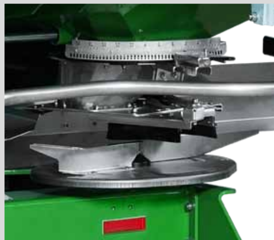
SOWING SYSTEM WITH VISIBLE SCALE AND BRUSHES
